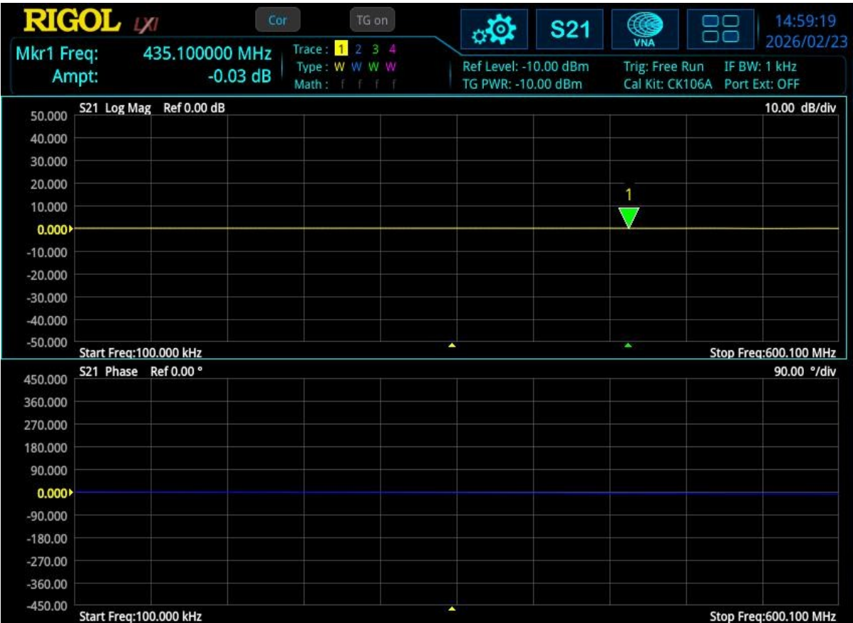
Figure 4: Insertion Loss vs Frequency
