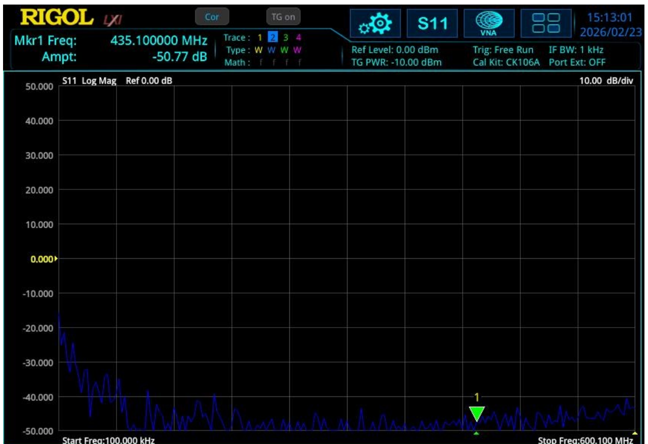
Figure 6: Return Loss vs Frequency
