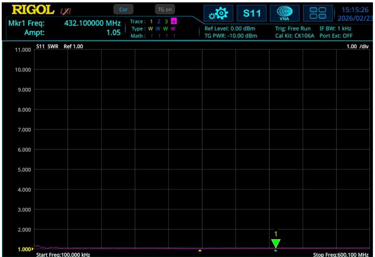
Figure 5: Standing Wave Ratio (SWR) vs Frequency
